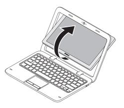
**2.** Push the display panel from the top and rotate it 180 degrees clockwise.
