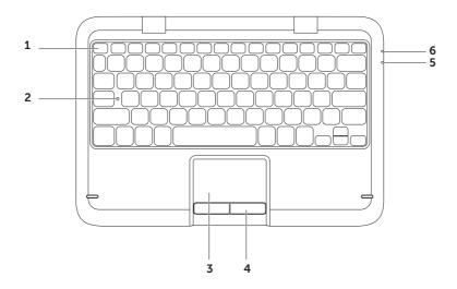
1 Function key row — The wireless enable or disable key (↑), brightness increase ♠ and decrease ♠ keys, multimedia keys, and the touch pad enable or disable key ♠ are located in this row.
